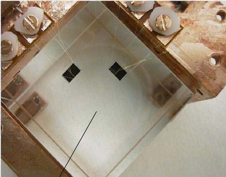
absorber crystal (Sapphire- or \text{CaWO}_4 )
