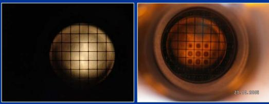
Polypropylene 15µm thick with strongback
