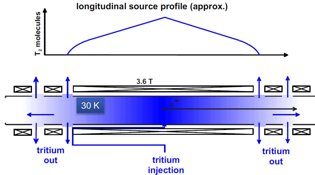
Parameters like temperature, tritium purity, injection pressure, ...
