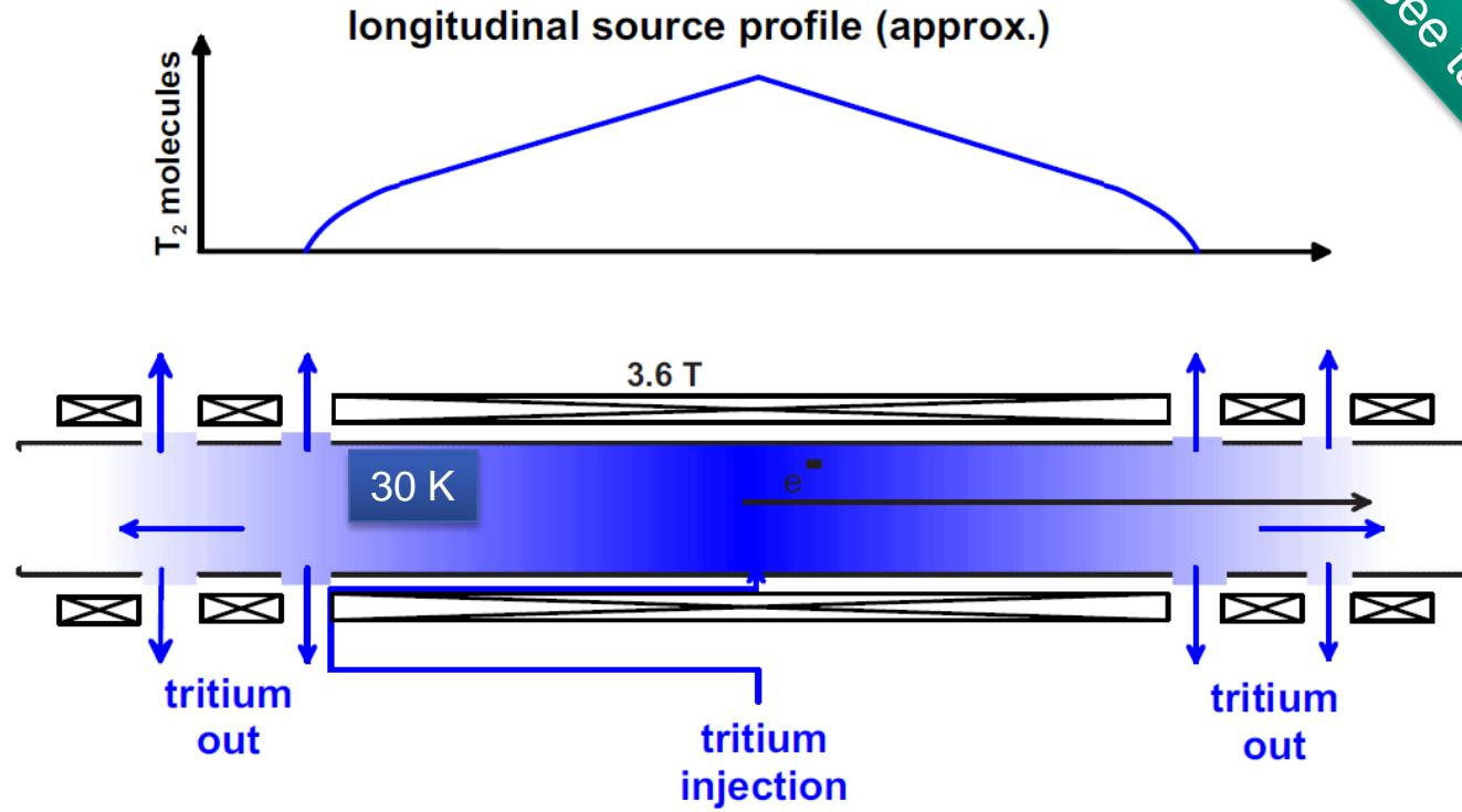
Parameters like temperature, tritium purity, injection pressure, ... have to be stabilised on a  $10^{-3}$  level.
